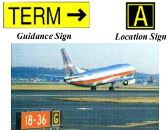
A driver would see these signs and markings when holding short of runway 18-36 at taxiway "G"
