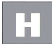
Helicopter Landing Area Marking
